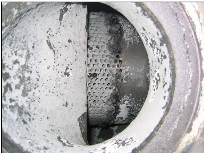
**Figure 3.** Level control valve on condensate outlet from Glycol settler. The salt is  $\text{NaHCO}_3$ .
